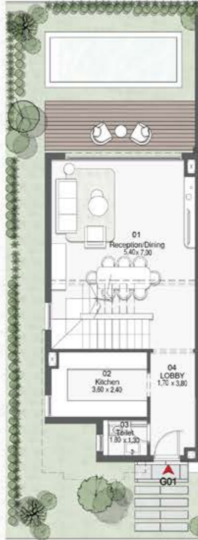
GROUND FLOOR FLOOR AREA = 67 M 2
