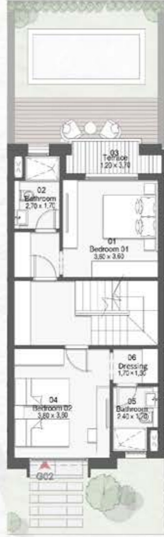
FIRST FLOOR FLOOR AREA = 63 M 2
